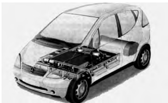
Figure 3.13 NECAR – Fuel cells in a Mercedes A-class
