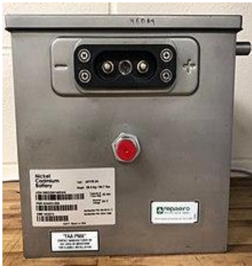
View of a vented cell aircraft battery from the side
